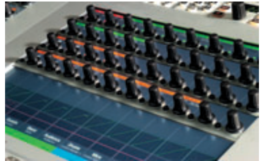
Vistonics® screen in channel bay
