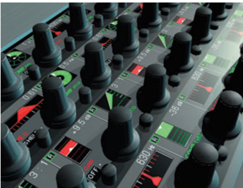
Vistonics: 40 rotary encoders and switches mounted on a TFT Screen
